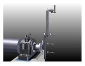
The Offset laser fixture is adjustable in a plane parallel to the flange face of the stationary machine and can be set at any position to eliminate the offset from the driven unit.
