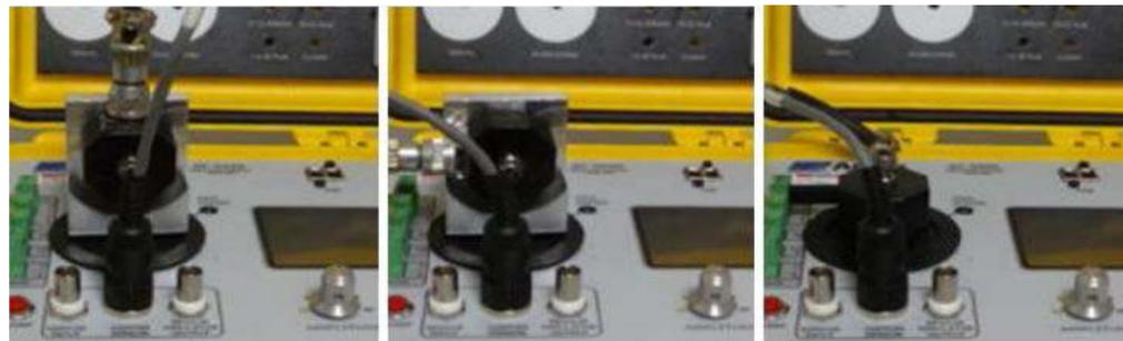
Figure 36. Sensor positioning and connection method
