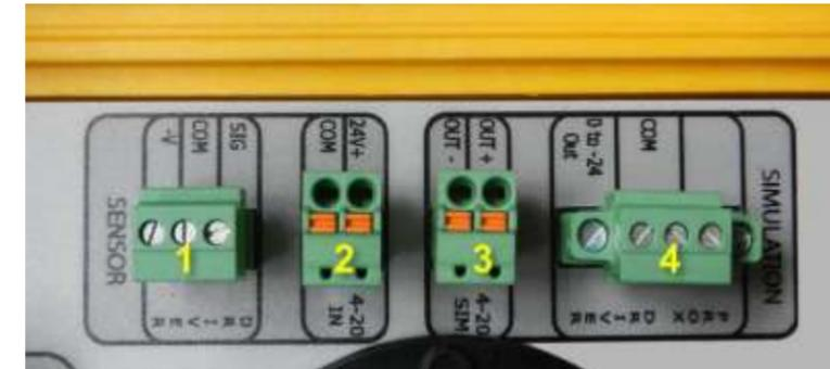
Figure 60. 4-20mA ("3") and proximity probe simulator connectors ("4")
