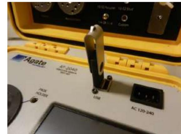
Figure 43. USB memory drive loaded in USB port
