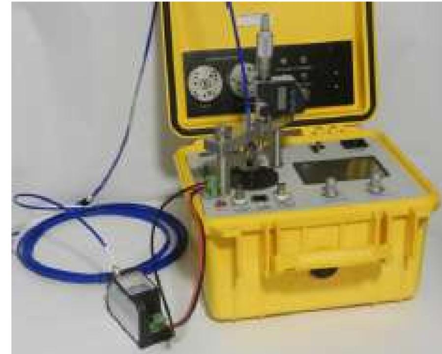
Figure 40. Proximity probe driver connected to AT2040
