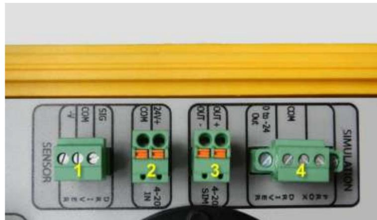
Figure 29. Connect the sensor to connector "2"
