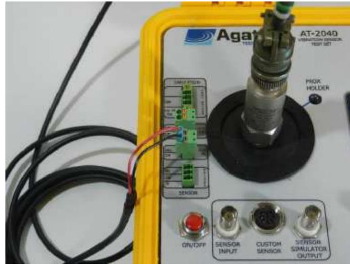
Figure 28. Sensor mounted to the AT2040
