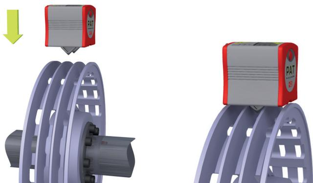
The Fixturlaser PAT units are very easily mounted on the pulleys. The spring action probe finds the center of the belt groove. The industrial built-in magnets snap the units to the pulley in a perfect fit.
